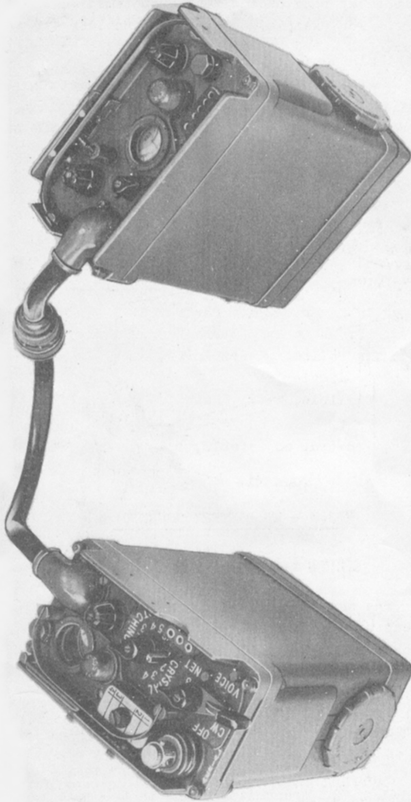
FIG. 2. TRANSMITTER, A510 AND RECEIVER, A510
